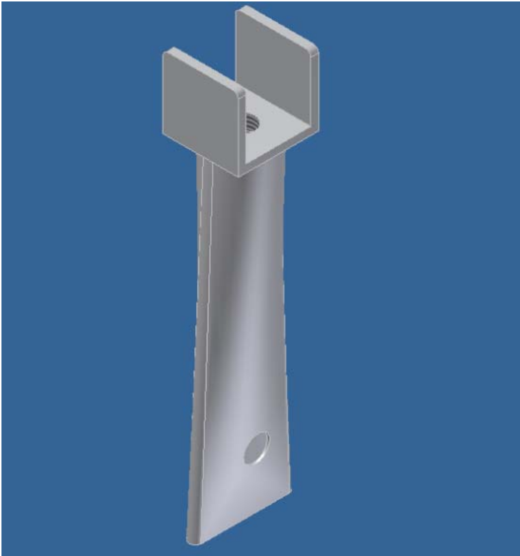
Figure 8A: Pictorial view of weeding-cone holder (standard)
