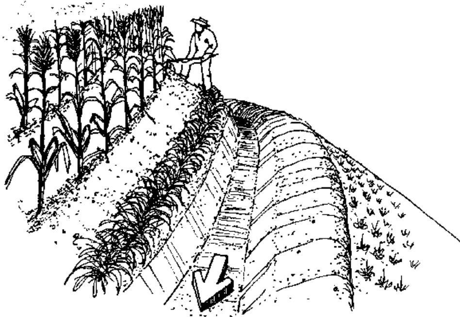
Fig. 11. Contour drainage ditch
